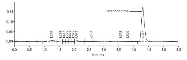
FIG. 2. Chromatogram of 9-methoxycanthin-6-one standard with retention time of 4,317 min
