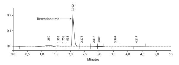
FIG. 1. Chromatogram of 9-hydroxycanthin-6-one standard with retention time of 2,092 min.
